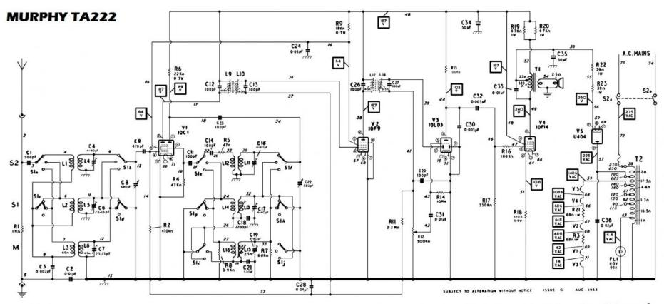
In later sets, R22 and R23 are deleted and replaced by one 1800, 6W, wire wound resistor Part No. 51082. This resistor is located on the top of the chassis in front of V5.
